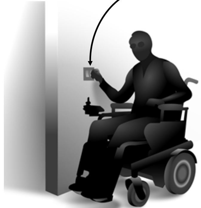
Universally designed accessible light switch mounted at 40"
